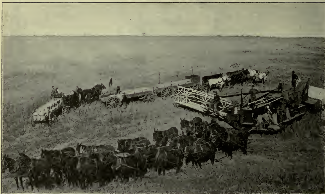
FIG. 278. — Cutting wheat in the fertile wheat region of eastern Washington. By this large machine, drawn by thirty-two mules and horses, the wheat is cut, threshed, and put into sacks ready for shipment.
